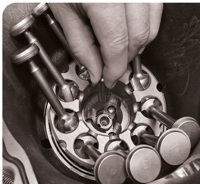
24. Assemble the support pin.
