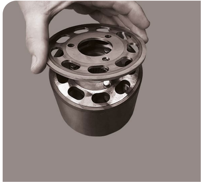
18. Remove the sliding plate.
