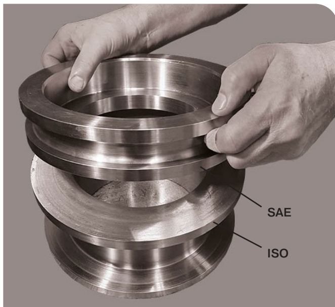
15. Choose the correct assembly tool for the bearing package, ISO or SAE.
