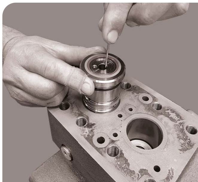
40. Locate and assemble the valve sleeve.
