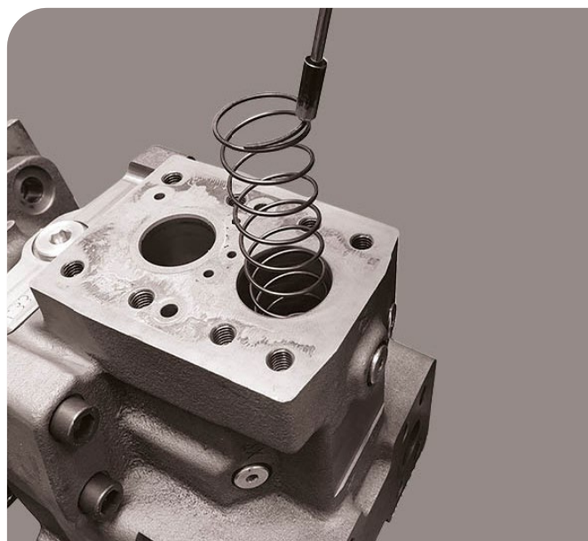
12. Remove the modulating spring.
