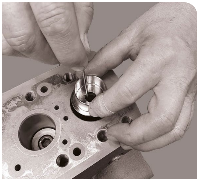
35. Locate and assemble the spring seat.
