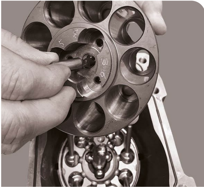
29. Assemble the support pin.
