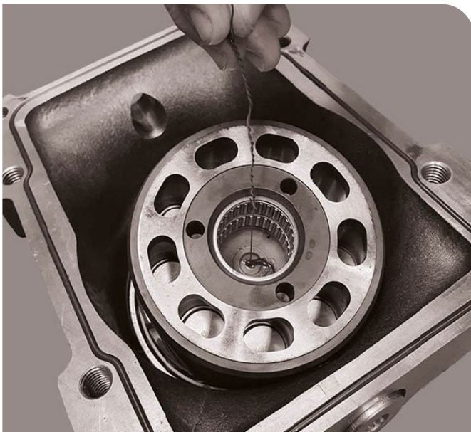
31. Make sure that the support pin is in correct position by using a thin steel wire. It should stop against the support pin. You can also see grease coming up from the centre hole in the cylinder barrel.
