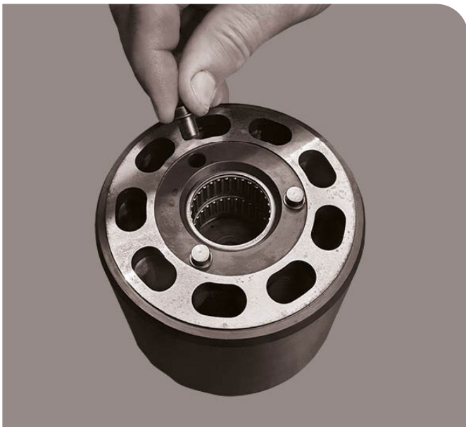
19. Remove the guide pins.
