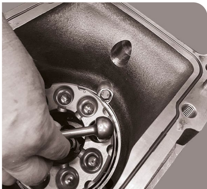
23. Assemble the pistons.
