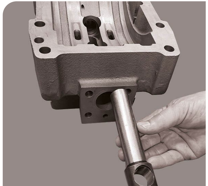
2. Assemble the setting piston
