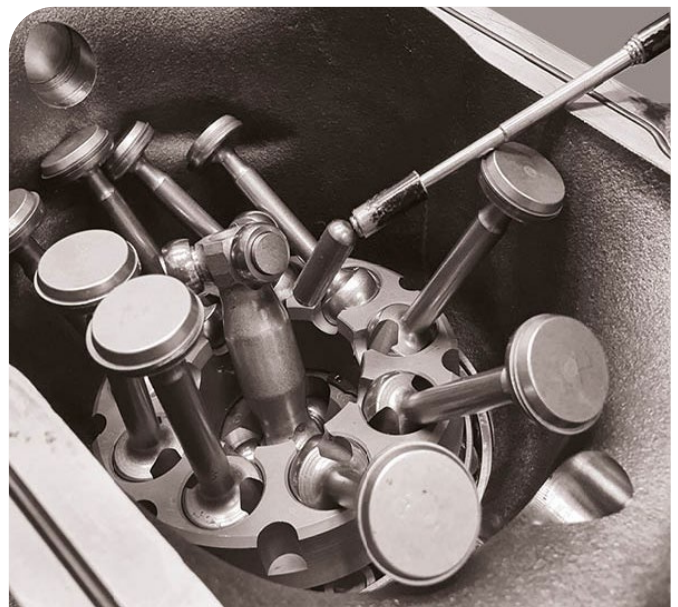
20. Remove the support pin that was assembled between cylinder barrel and joint shaft. Locate it and use a magnet to pick it up.
