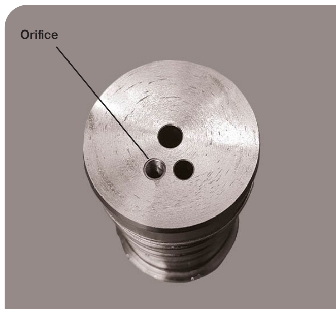
10. Remove the orifice.
