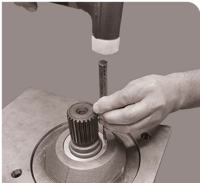
21. Fit the support ring and carefully tap down the shaft seal and support ring.
