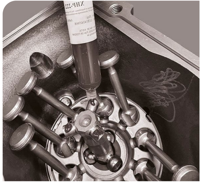
26. Put grease on the joint shaft.
