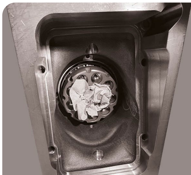
28. Protect the ball sockets in the shaft with some paper or a cloth before you press out the bearing package.
