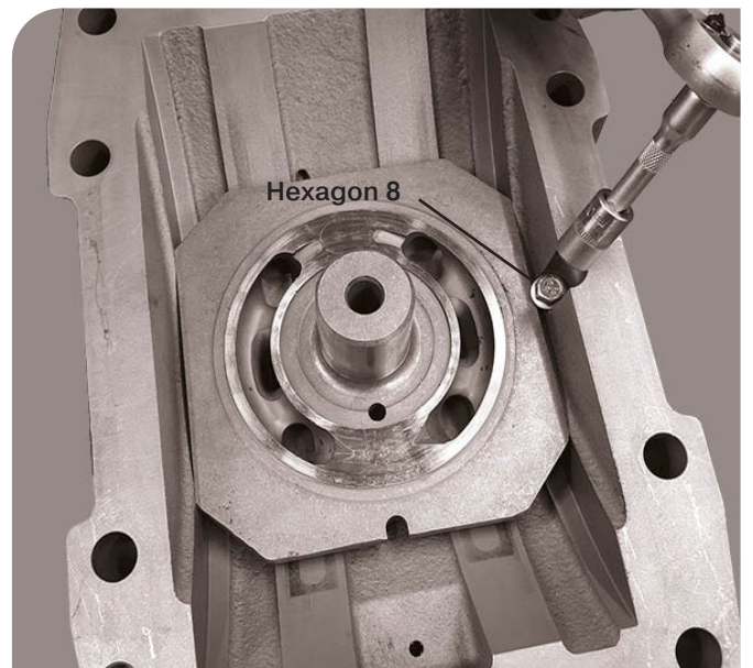
36. Disassemble the hexagon screw.
