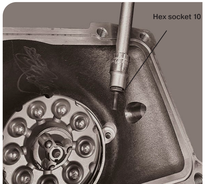
24. Disassemble the hexagon screw.
