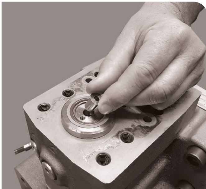
3. Remove the spacer
