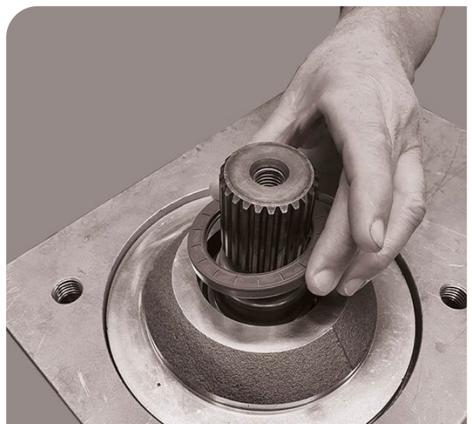
20. Fit the new shaft seal, be careful so the sealing surface isn't damaged.
