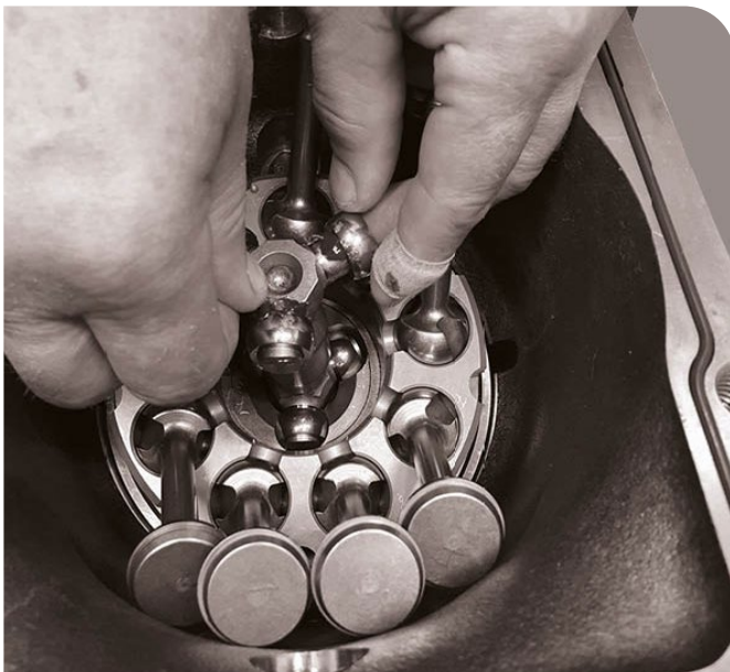
27. Assemble the rollers, grease is needed to keep them in place.
