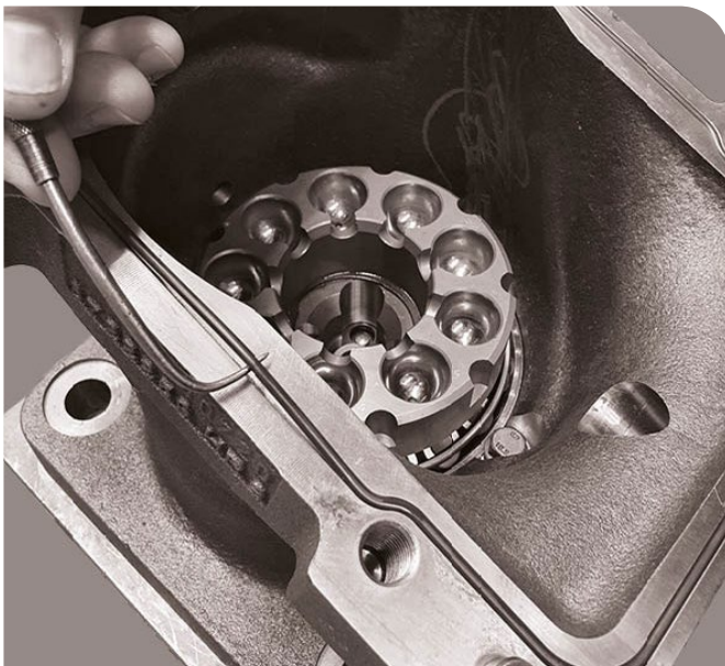
23. Disassemble the o-ring.
