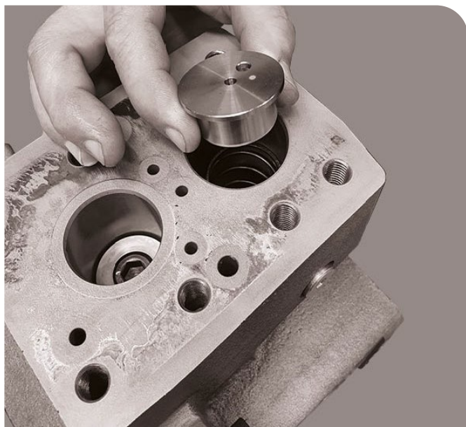
39. Assemble the spring seat.
