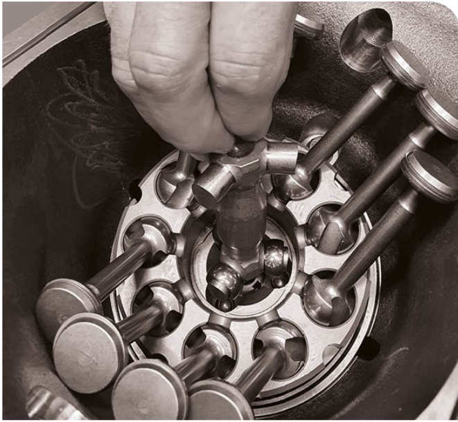
25. Assemble the joint shaft with the first 3 rollers.
