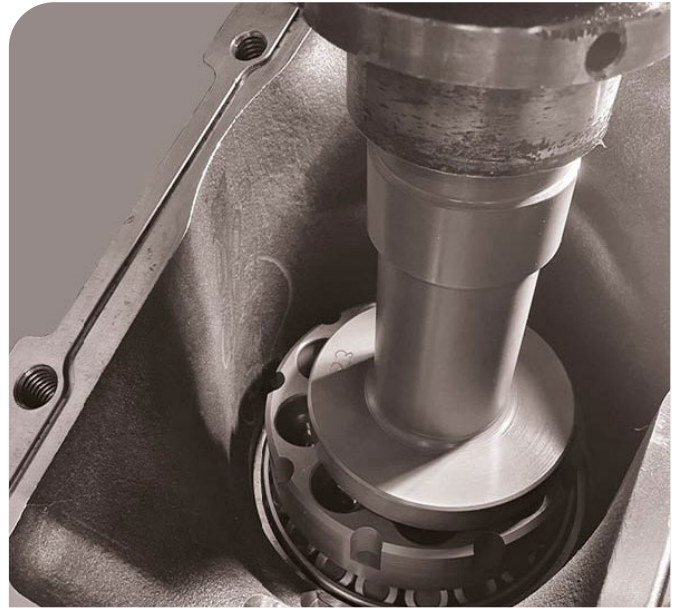
18. Use a press and press down the bearing package.
